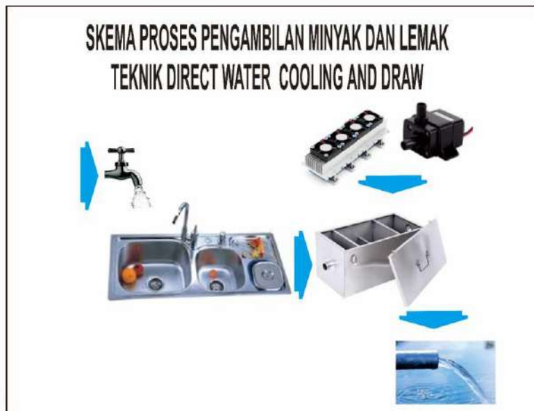
Desain Grease and Oil Catcher teknologi direct water cooling and draw
