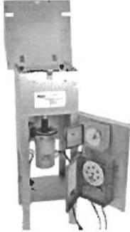
The Tisch Environmental TE-5170V is a total suspended particulate, high volume air sampler. The TE-5170V uses a volumetric flow controller (VFC) to maintain a constant volumetric flow rate during sampling. It is available with a brushless or brush style motor and your choice of a 7-day mechanical timer or a US EPA recommended digital timer.
